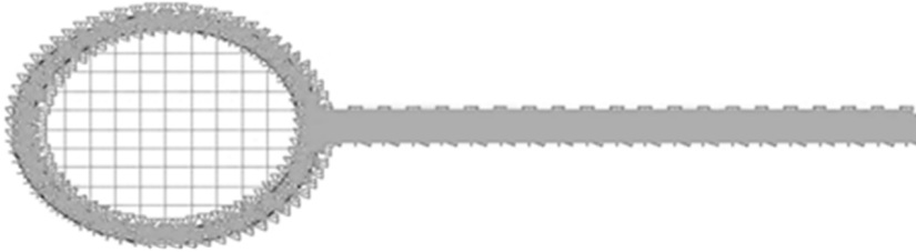
Fig. 3. Finite element model of badminton racket modified by Domain Superposition Technique
